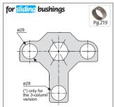
The side pre-holes must be made in the extruded part as shown in the diagram, to create the housing of the anti-friction bushings for the guides with 2 and 3 ø25 columns. A hole must be made at the base of the extruded part for the version with 3 columns.
