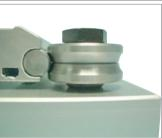
Fig.2: The new rollers with a gothic arch profile quarantee wider contact surfaces than traditional rollers with a V-shaped profile. This reduces the contact pressures and increases the applicable loads, reliability and durability.
