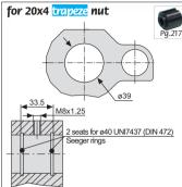
2 seats must be made for ø40 Seeger rings at the indicated distance for the axial block; a seat must be made for an M8 threaded grub screw for anti-rotation.
