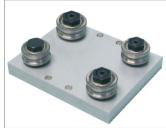
Fig.1: The new 308-type carriage does not have spotfacings on the upper part, for the screws that fasten the rollers. The latter are fitted by tightening them on the lower side making it easier to clean the carriage. The pre-load is adjusted by acting on the two eccentric rollers, like for traditional carriages.
